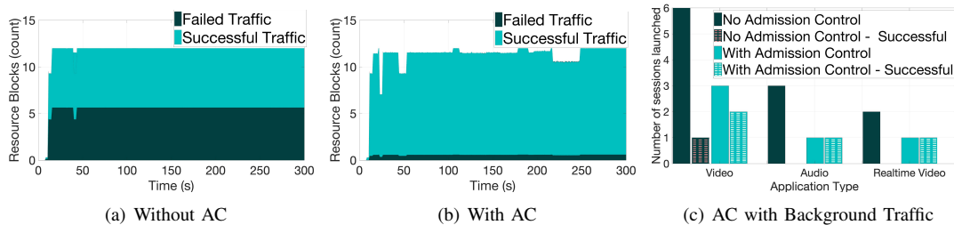
Fig. 1: (a) Without a resource-aware Admission Control (AC) algorithm, almost half of the LTE network’s resources are expended in failed sessions. (b) With the AC in place, this is reduced to \sim 5\% while preserving high network utilization and (c) most performance guarantees are met even in the presence of uncontrolled background traffic.
