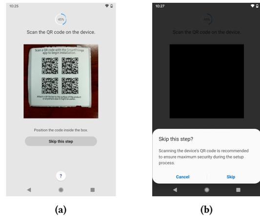
**Figure 11: Screenshots from the SmartThings smartphone application [28] that show (a) the commissioning of a Zigbee 3.0 device by scanning its QR code and (b) the warning message that is displayed when a user tries to skip this step.**
