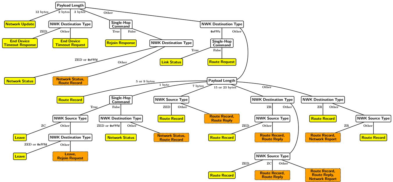
Figure 12: The decision tree that we developed for the identification of encrypted NWK commands based on the assumptions that we stated in Sections 3 and 7.2 as well as the reconnaissance attacks that we presented in Section 7.1. Pure leaf nodes are colored yellow with a solid outline, while impure leaf nodes are colored orange with a dashed outline.
