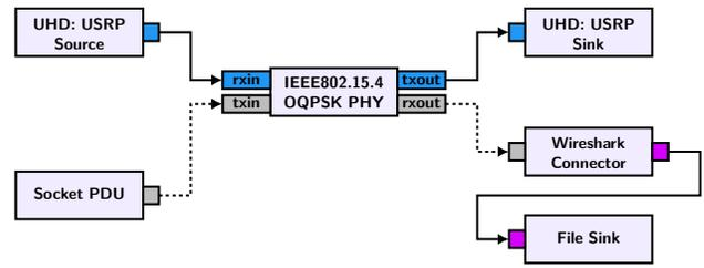
Figure 5: A simplified GNU Radio Companion flow graph that uses an implementation of the IEEE 802.15.4 O-QPSK PHY layer [7] to transmit and receive Zigbee packets.
