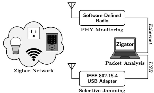
Figure 1: Zigator analyzes captured Zigbee packets to enable the development of selective jamming and spoofing attacks with an IEEE 802.15.4 USB adapter, which we study by capturing I/Q signals with a software-defined radio.
