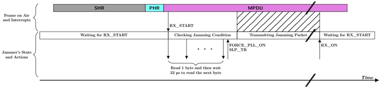
Figure 6: Our selective jammer provides fine-grained control over the jamming condition by reading the bytes of a transmitted packet as they are being received to determine whether it will be jammed or not before the completion of its transmission.
