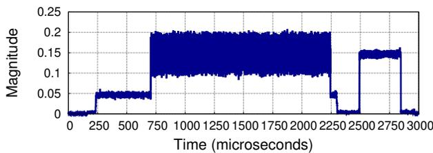
Figure 7: Captured I/Q signal during the selective jamming of a Zigbee packet and injection of a MAC acknowledgment.
