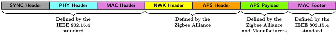
**Figure 2: High-level view of a general Zigbee packet without any Auxiliary Header or any Message Integrity Code.**
