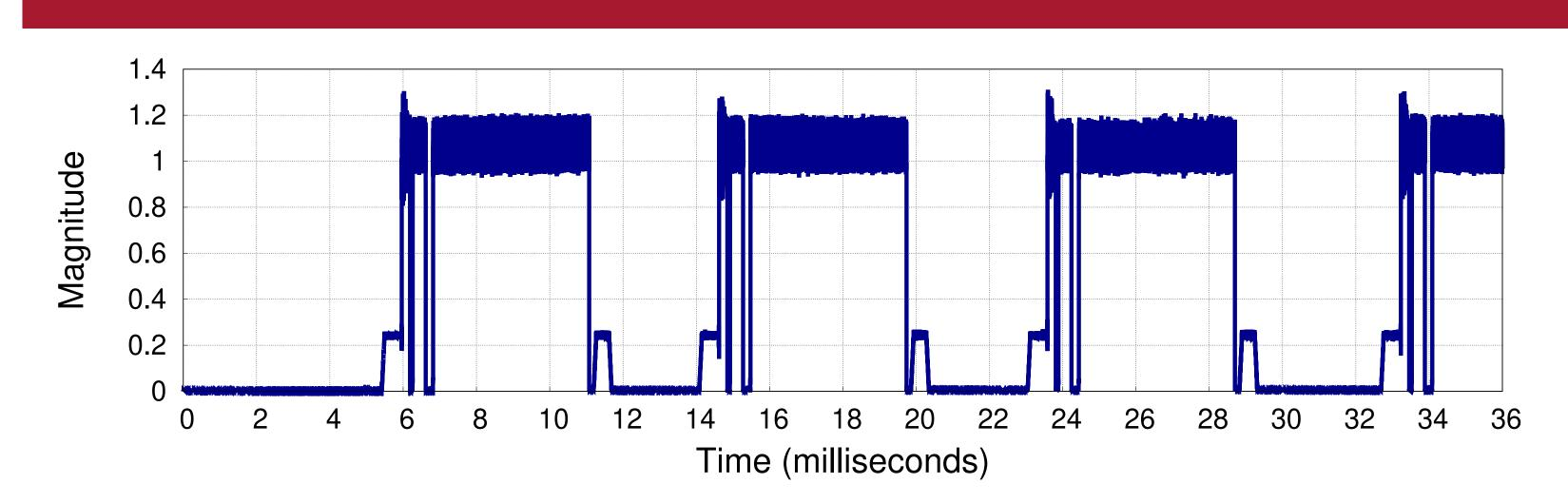
We developed an energy depletion attack that exploits the way that Zigbee devices are currently handling *Data Requests* by selectively jamming them and injecting spoofed packets [1]
